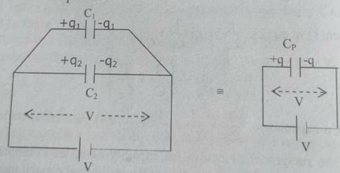
Consider two capacitors of capacitance C1 and C2 connected in parallel. Let V be the potential difference across each capacitor or combination and q1 and q2 be their charges respectively.
